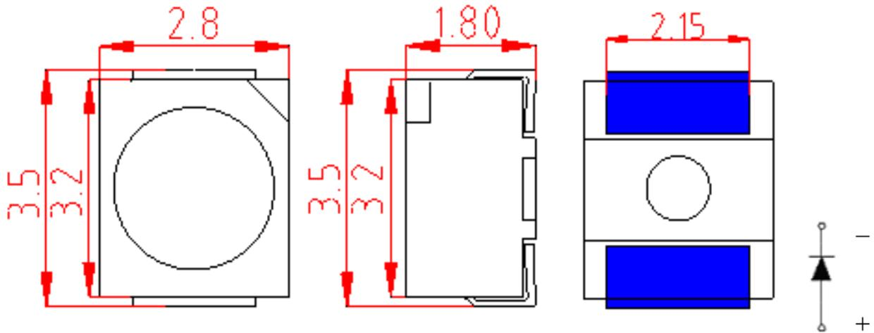
Notice: Tolerance of measurement of Dimension:  $\pm 0.2\text{mm}$
