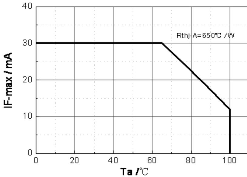
Figure4. Forward Current VS. Ambient Temperature
