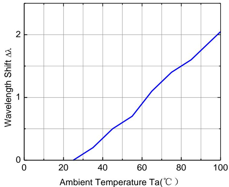
Figure2. Wavelength Shift VS. Ambient Temperature
