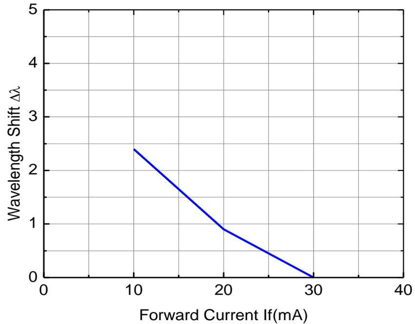
Figure5. Wavelength Shift VS. Forward Current
