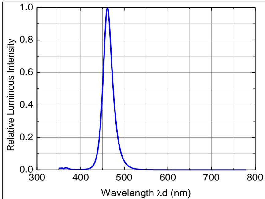
Figure7. Spectral Power Distribution VS. Wavelength
