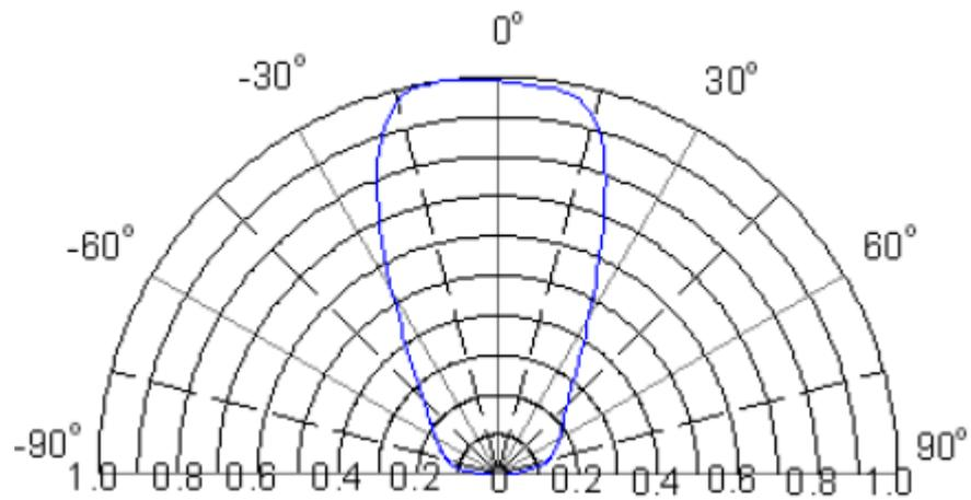
Figure6. Relative Luminosity VS. View Angle
