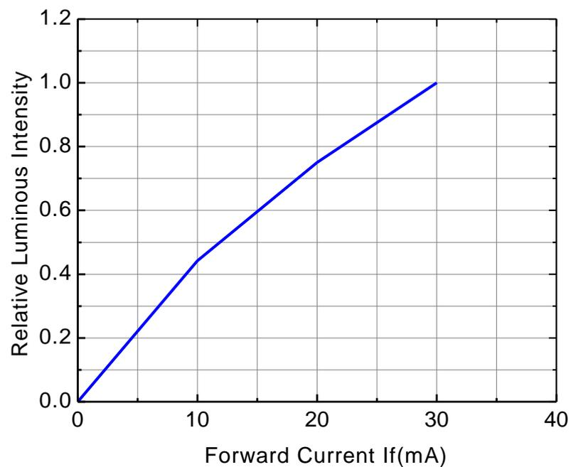
Figure8. Relative Luminous Intensity VS. Forward Current
