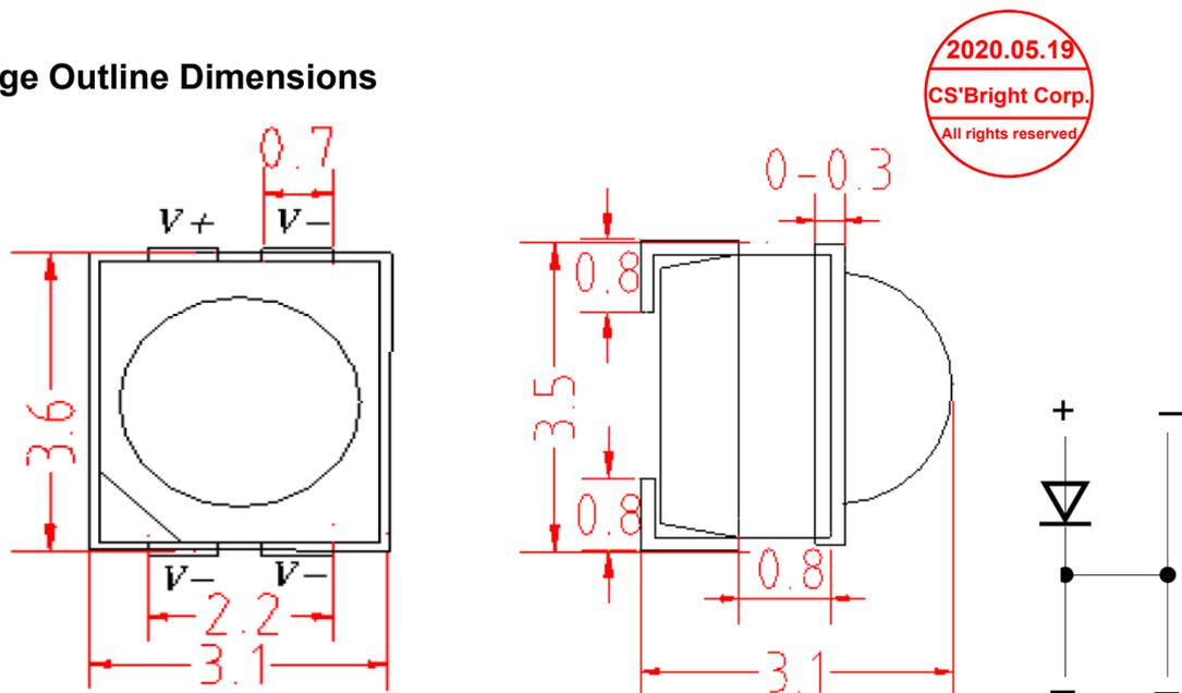
Notice: Tolerance of measurement of Dimension:  $\pm 0.2\text{mm}$
