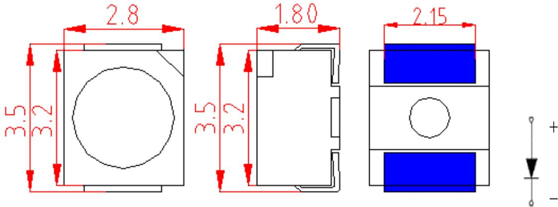
Notice: Tolerance of measurement of Dimension:  $\pm 0.2\text{mm}$
