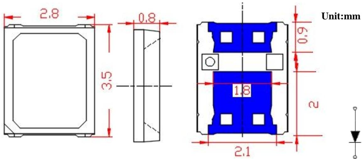
Notice: Tolerance of measurement of Dimension:  $\pm 0.2\text{mm}$
