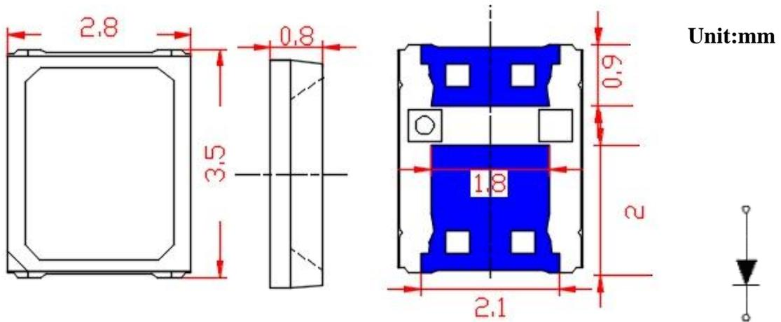
Notice: Tolerance of measurement of Dimension:  $\pm 0.2\text{mm}$
